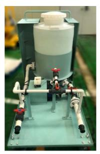
Hi-ACE removes SCALE deposited in the electrolyzer effectively and can maintain the electrolyzer condition as good.
